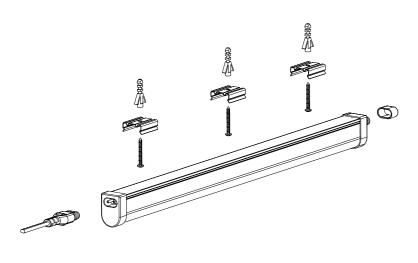
Step 1. Maka right position and screw hole on the ceiling, screw the clip on the ceiling tightly.
